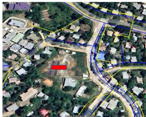
Figure 11. Naha Residential area sewage pipeline distribution
